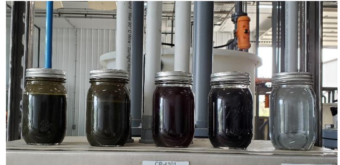
Samples of processed manure through NCS. Raw manure is on the left. Clean water is on the right.
