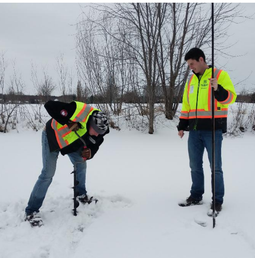
Fitchburg employees core through the ice at one of the city's water quality ponds to measure the depth of water and soft sediment. When there is less than 3.5 feet of water, dredging is done to remove buildup, which helps ensure the ponds can effectively clean water by allowing suspended solids (including attached phosphorous) to settle out.
