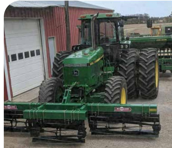
*This front-mounted roller crimper allows for simultaneous flattening of a cover crop while planting a new cash crop.*
